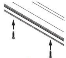
Pre-drill 7mm holes on the aluminum profile, secure the profile with screws on the surface, the height of the screw head shall not exceed 2mm.
